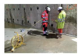
The **SixGyro gyroscopic probe** provides **borehole deviation measurements** regardless of whether they are horizontal or vertical to **any depth / length.**
